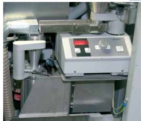
Integral laser granulometer for fineness analysis of cement or raw meal samples.
