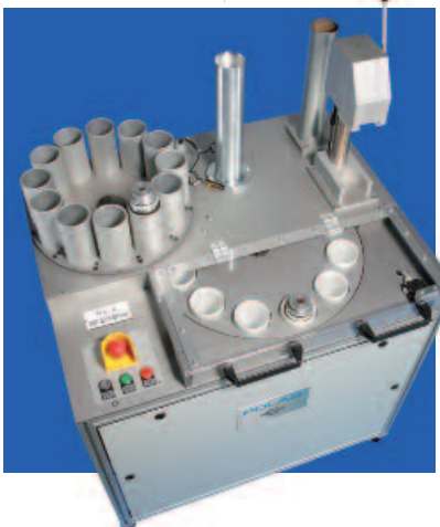
Semi-automatic pneumatic delivery receiving station with magazines for received and empty capsules.
