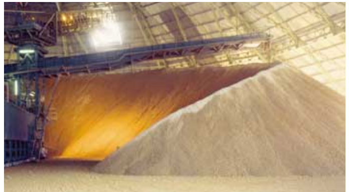
Material discharge via the central column.
