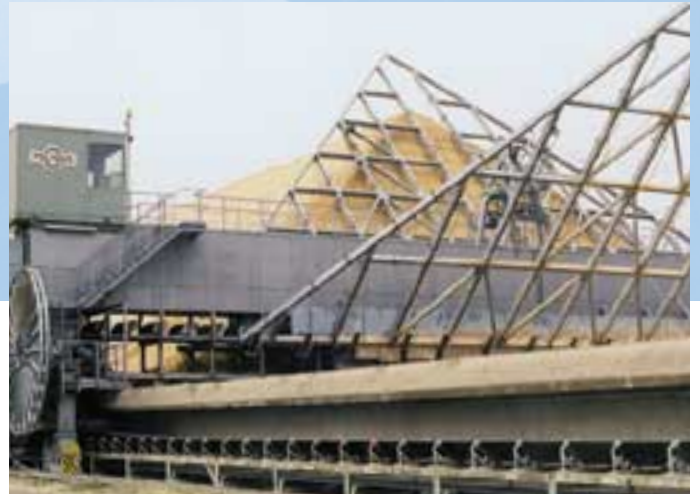
Polysius bridge scrapers have span widths of up to 55 m and reclaiming capacities of up to 1,500 tph.
