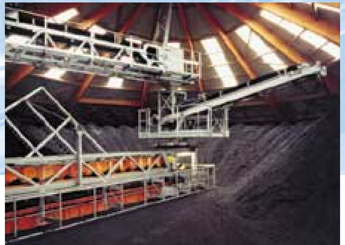
Coal stockpile with cone-shell stacking method. The smallest stockpile so far installed: diameter only 25 m.
