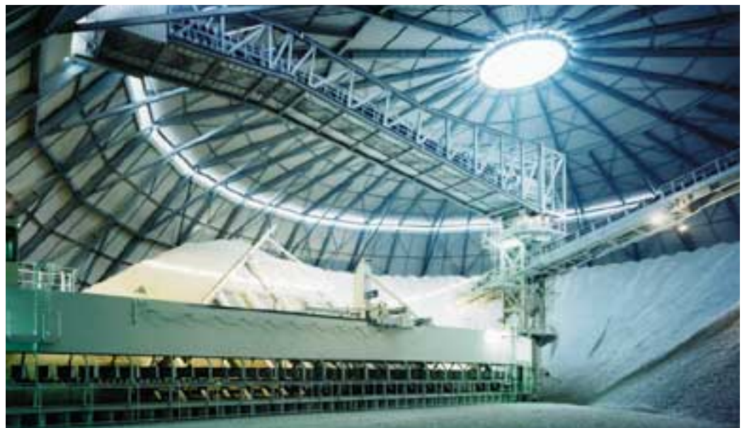
Coal stockpile with cone-shell stacking method. The smallest stockpile so far installed: diameter only 25 m.
