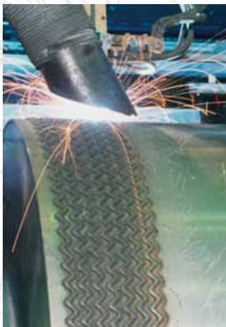
The profiles welded onto the grinding rolls maximise the feed material pull-in capability and minimise the relative movement between the material being ground and the roll surface.
