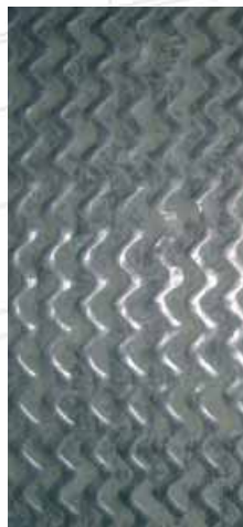
The profiles welded onto the grinding rolls maximise the feed material pull-in capability and minimise the relative movement between the material being ground and the roll surface.
