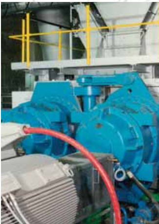
Drive system: planetary gear unit with electric motors (constant or variable speed).
