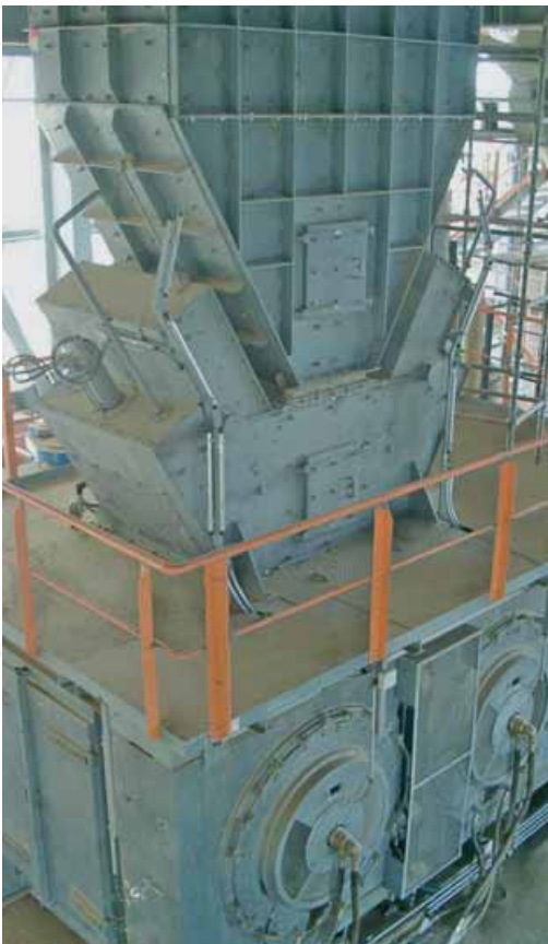
POLYCOM® for clinker grinding in a combi grinding system in Saudi Arabia.
