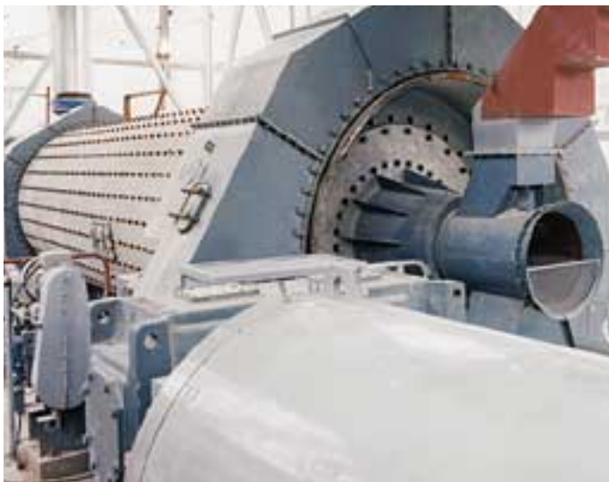
Tube mill with direct drive.
