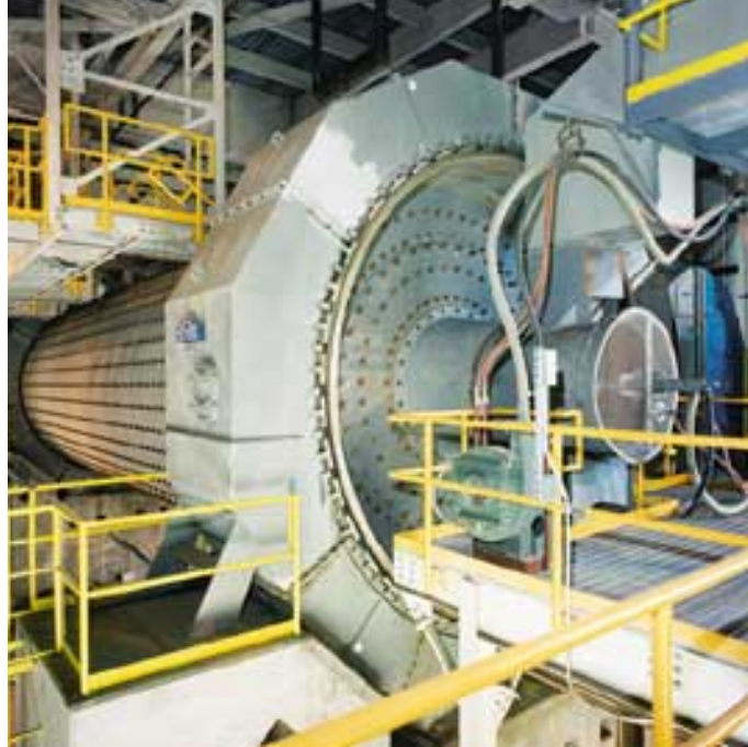
Two-compartment separator mill for cement clinker grinding in Florida, USA.
