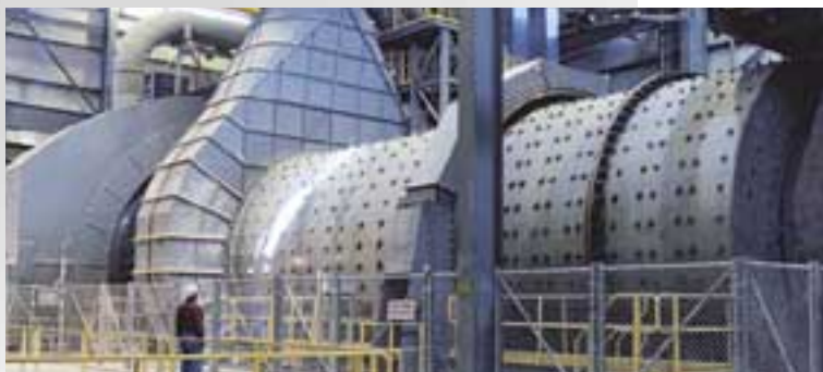
6.2 m x 25.5 m DOUBLE ROTATOR® equipped with 11,200 kW ring motor for gold ore comminution in the USA.
