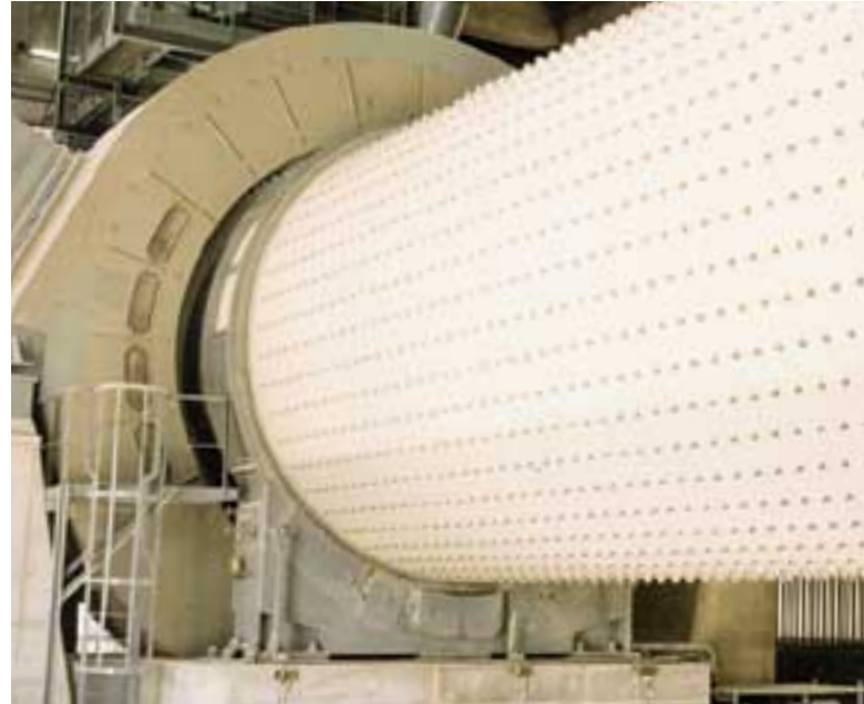
Tube mill with ring motor.
