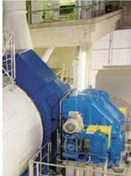
Tube mill with COMBIFLEX® drive unit.
