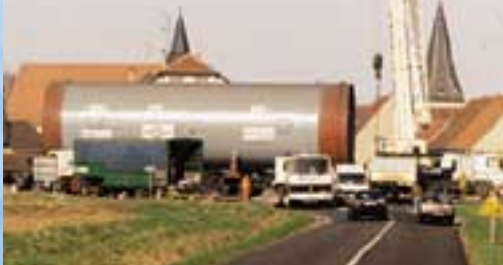
A 6.2 m x 20 m mill shell on its way from France to Malaysia.
