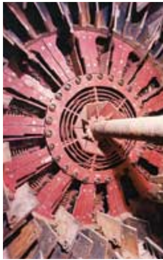
View into the drying chamber of a DOUBLE ROTATOR®.
