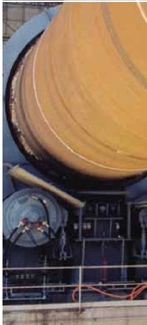
POLRO® two support kiln for a cement clinker output of 4,900 tpd in Australia.
