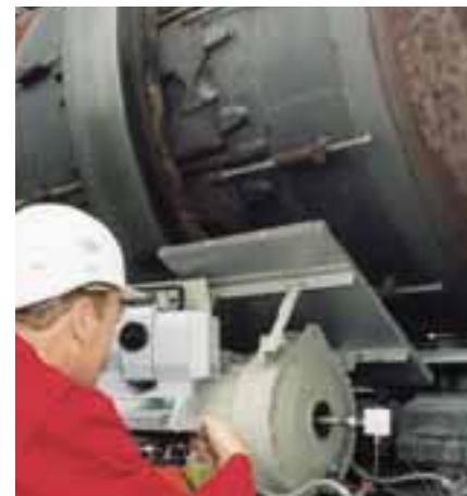
POLSCAN® measurement of a rotary kiln.
