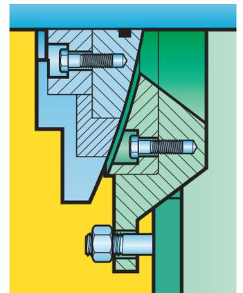
Practical experience has shown that it is possible to adjust the seal gap to less than 1 mm, which minimises the inleakage of false air, even in long-term operation.
